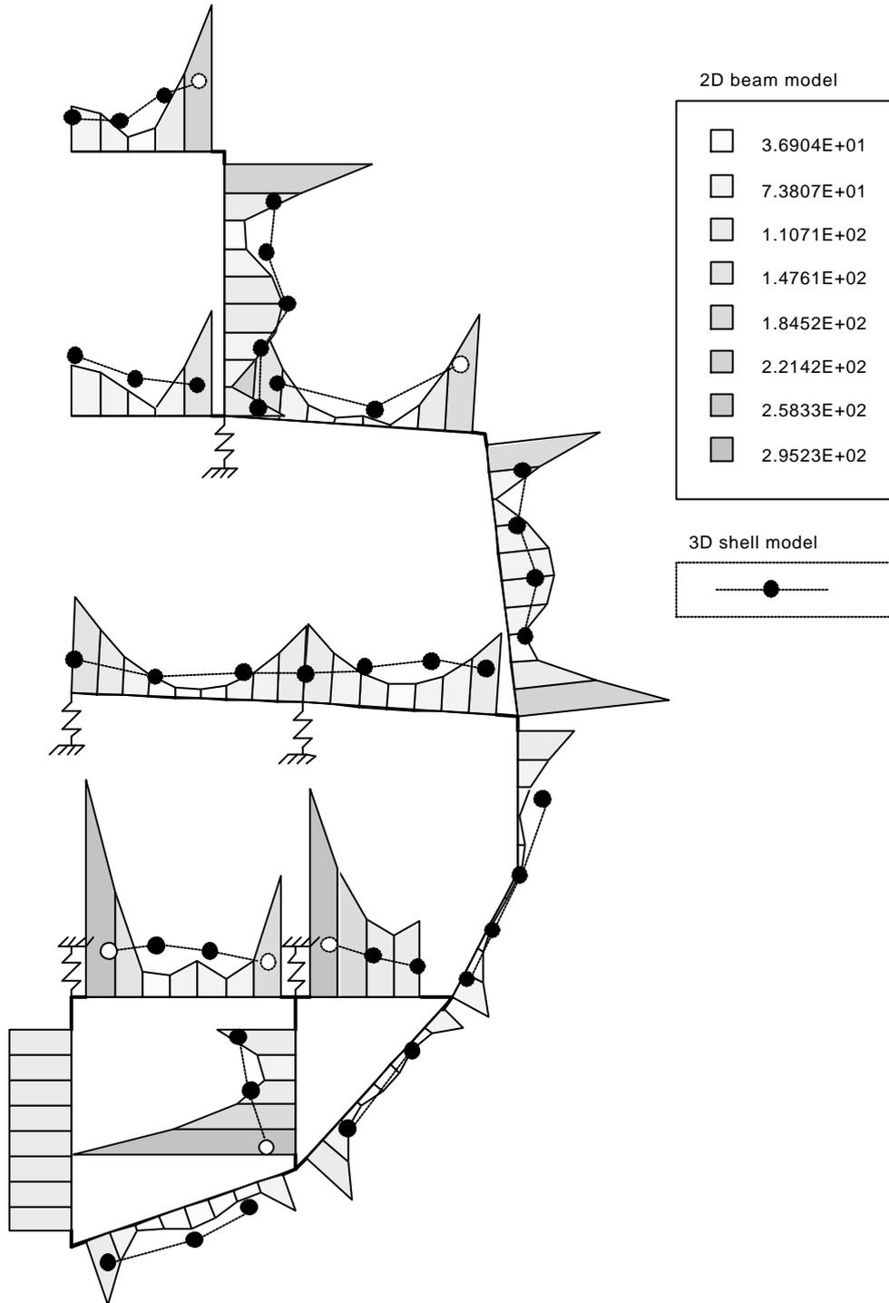
Figure 11 – Von Mises Stress at flange frame location
