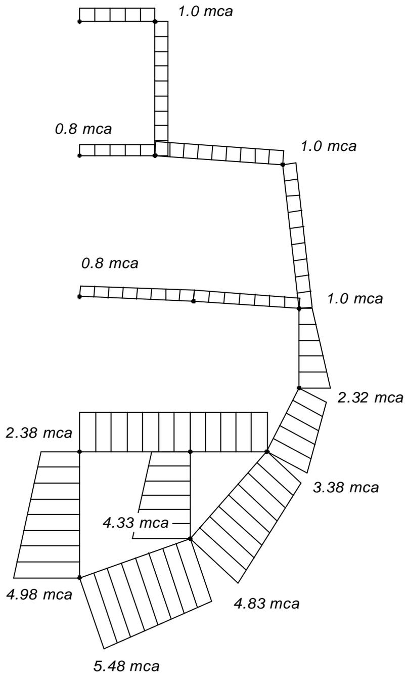
Figure 6 – Hydrostatic load used on the three dimensional model
