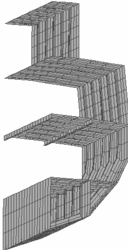
Figure 7 – Three dimensional model using shell elements
