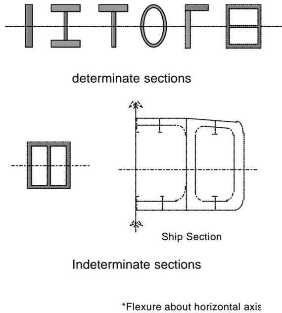
Figure 3 – Examples of beam cross sections
