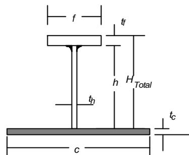
Figure 9 – Beam cross section characteristics
